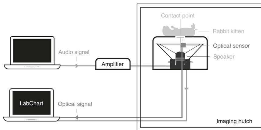
**Fig. 2 Set-up of the vibrotactile stimulation device.** The device consists of an amplifier and a metal box with a speaker and optical sensor inside. A rod is connected to the conus of the speaker which transmits the vibration of the conus to the skin of the kitten.
