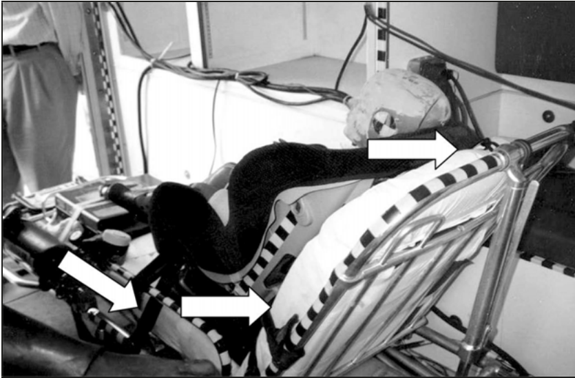
Two horizontally oriented belt paths and one vertical belt path for securing the car safety seat to a stretcher. (Photo, EMS Safety Foundation, Nadine Levick, MD, MPH)
